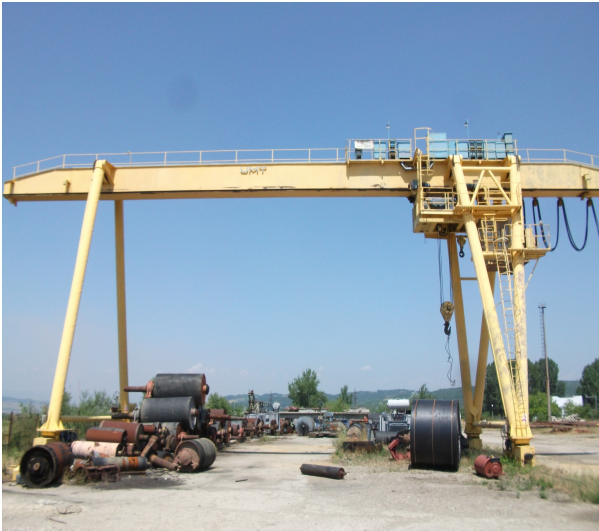
Figure 1. MPT 20/5 gantry crane
